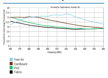
All graphs are generated under laboratory conditions. Real-life performance may vary. Reader power: 29 dBm. Antenna sensitivity: -70 dBm
