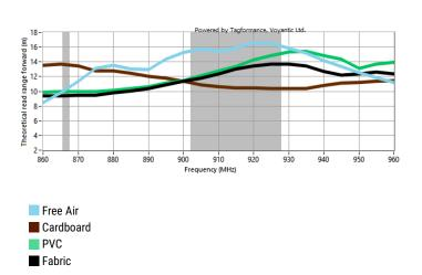
All graphs are generated under laboratory conditions. Real-life performance may vary. Reader power : 29 dBm. Antenna sensitivity : -70 dBm
