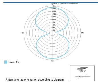
All graphs are generated under laboratory conditions. Real-life performance may vary. Reader power : 29 dBm. Antenna sensitivity : -70 dBm
