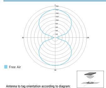
All graphs are generated under laboratory conditions. Real-life performance may vary. Reader power: 29 dBm. Antenna sensitivity: -70 dBm
