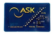
All contactless system installation, tuning, or diagnostic, require a tool to measure the radio field performance.
